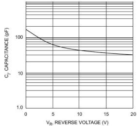
Fig. 3 Typ. Junction Capacitance vs Reverse Voltage
